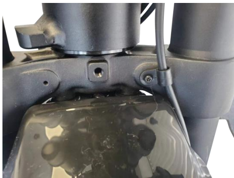
Front fender and rear shock absorber zip tie demonstration illustrations.
