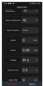
State Of System: The system state will display the bike's condition in real time. Under normal circumstances, it will show "normal". In abnormal situations, it will display the corresponding fault information. When the bike malfunctions, please check the this state immediately.
